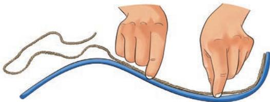
Fig. 5.8: Measuring the length of a curved line
